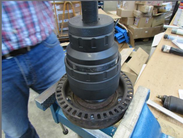
5. Then brace the pull-off adapter on the bearing cup, where you screw the pull-off tool housing and the pressure sleeve fixed with the ring spanner.
