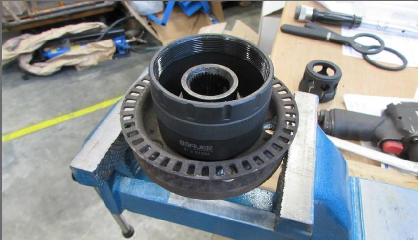
2. Select the matching pull-off adapter and place it as close as possible to the flush joint of the bearing cup.
