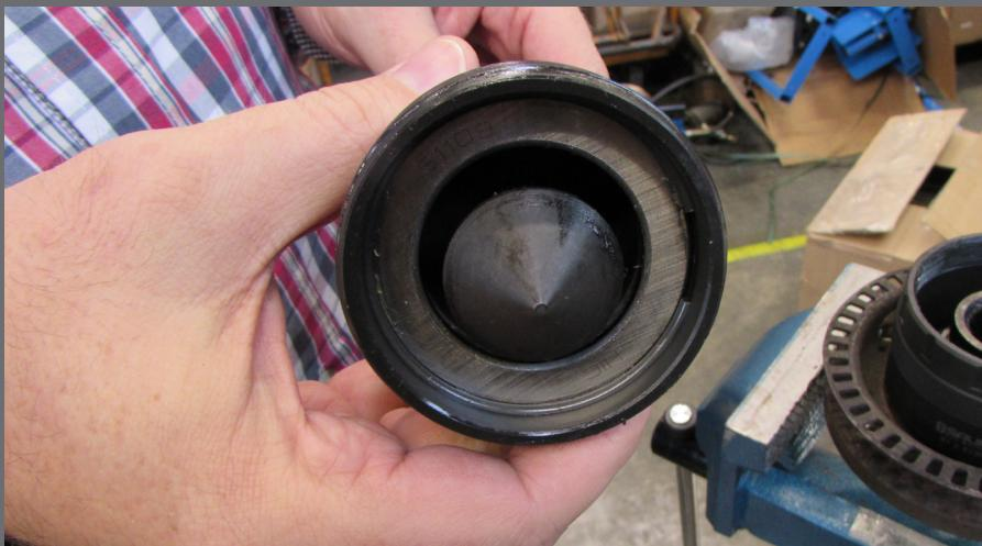
4. Screw the pull-off tool housing into the external pressure sleeve.
